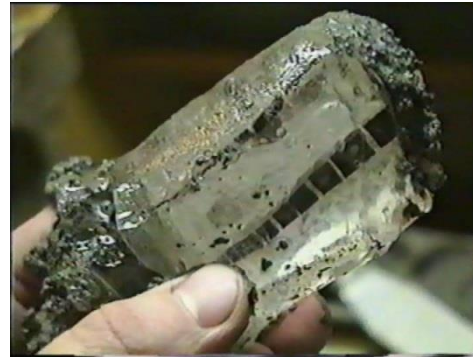
Core from subaquatic permafrost
