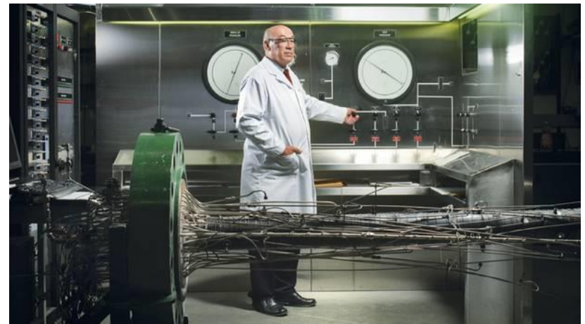
Combustion tube for laboratory experiments
