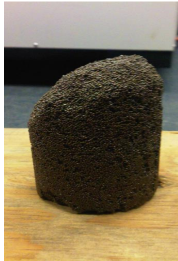
Rock sample after shearing
